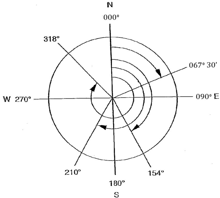
**WRITING BEARINGS** – Turn East or West from the N-S line to a maximum of 90°. The bearing value always has an N or S prefix and an E or W suffix. Use two digits for degrees, e.g., N 06° W. Use two digits for non-zero minutes and seconds. Must have minutes if you have seconds, even if 00'.
